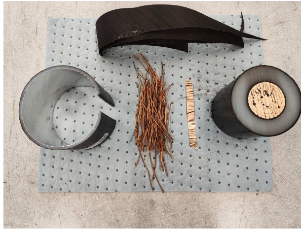
Figure 4.2: Picture showing the sample and everything that was removed during the first step of the sample preparation process. The sample, which is now ready for having electrodes applied if the OSL is to be studied, can be seen on the right. The removed swelling bands (top), protective sheath (right), and copper wires (middle) can also be seen.
